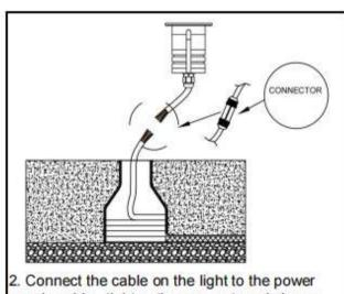
Connect the cable on the light to the power supply cable, tighten the connector, pls leave some length for future maintainance
